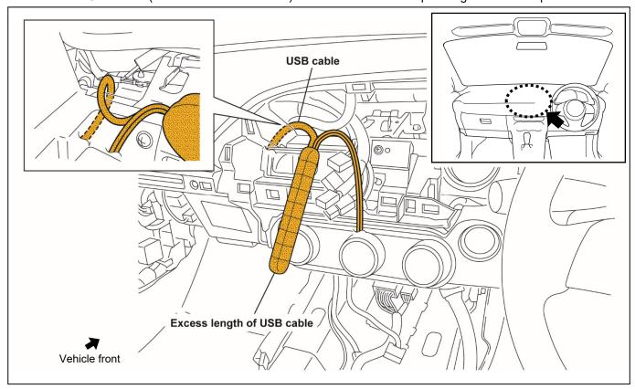
2. Route the USB cable to the underside of the front console.
