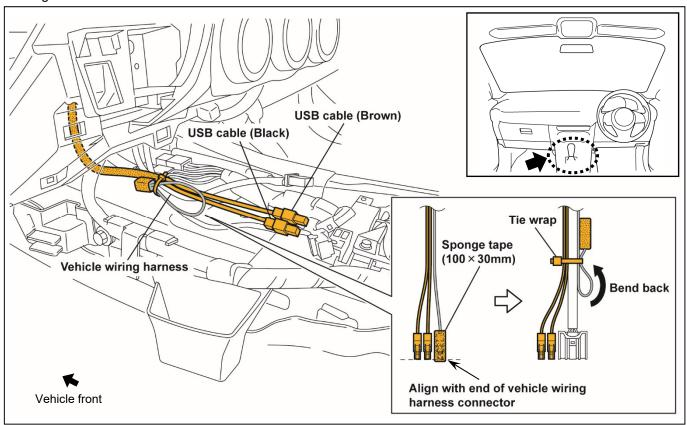
6. Push the excess length of USB cable under the dashboard member.
