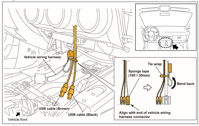
5. Push the excess length of USB cable under the dashboard member.
